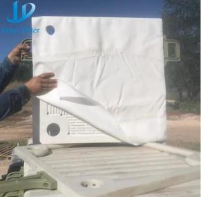
The filter plate and filter plate are arranged in order, the filter cloth is hung on the filter plate.
